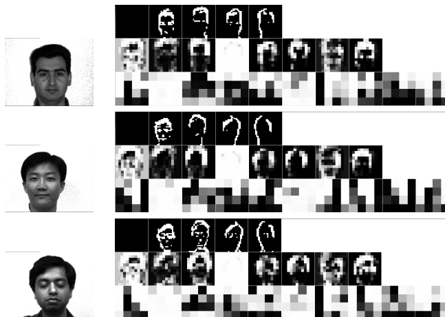
Fig. 1: Convolutional outputs for three images. Left shows three faces. Right shows filter outputs for each face image. Rows represent layers.
