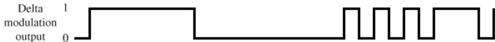
Figure 6.18 Example of Delta Modulation
