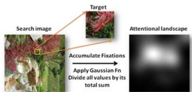
Figure 1. Computation process for attentional landscapes. After accumulating fixations from all subjects, we apply a 2D Gaussian function. The attentional landscape is normalized as probability density function.
