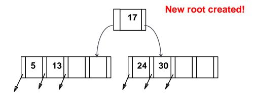
Note that 17 is "pushed up"; contrast this with "copy-up" for leaf nodes Push up: deletes key from lower level and inserts it in upper level
