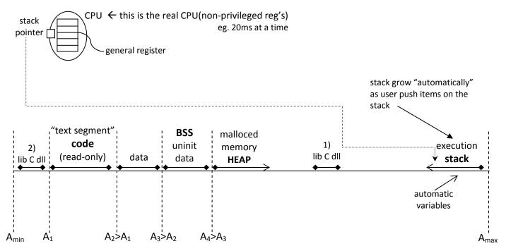
This is a flat address space, and all current systems use byte addressing. Here each byte of memory usable by the program running in the process gets its own unique address between  $A_{min}$  and  $A_{max}$ . Another process running at the same time sees its own private version of the address space.
