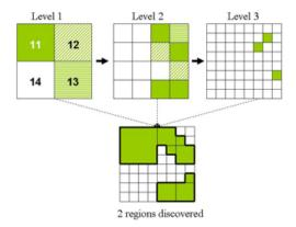
Fig. 3 Runing the SCMRG algorithm on a sample dataset
