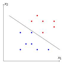
If S is linearly separable there are, in general, infinitely many hyperplanes that can do the separation.
