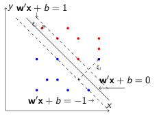
A vector  $\mathbf{x}_i$  is an outlier if  $\mathbf{x}_i$  is not positioned correctly on the side of the appropriate hyperplane.
