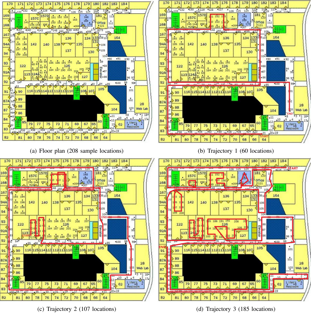
Fig. 1. Floor plan (68m \times 63m) with 208 sample locations, each represented by a black dot. The hallways are marked with white color and stairs with green. Black and blue areas are not penetrable. Three trajectories of different patterns and path lengths are shown in red color.
