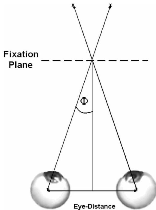
Figure 1. The definition of the vergence angle  $\Phi$ .
