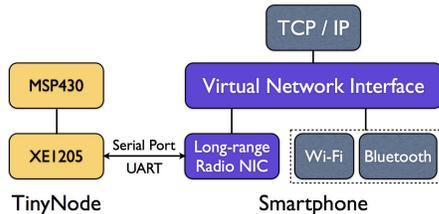
Fig. 3: Software Architecture
