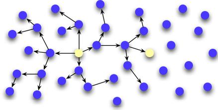
Fig. 1: Traditional Path Establishment (TTL=4)
