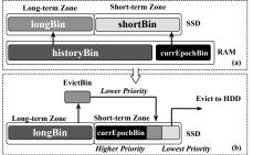
Fig. 4. High level idea of GREM: (a) cache admission and (b) cache eviction.
