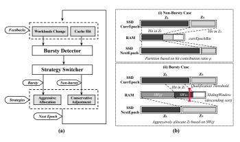
Fig. 5. (a) The high level sketch of D\_GREM. (b) Dynamic partition of  $Z_L$  and  $Z_S$  of D\_GREM.
