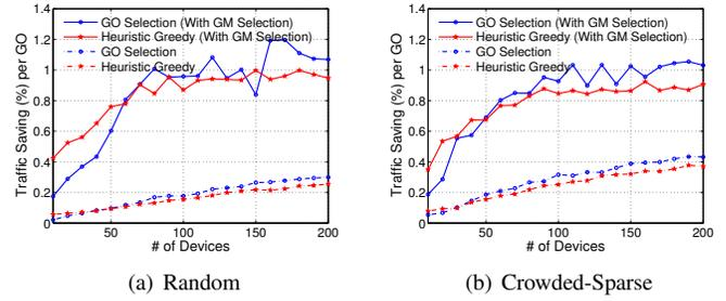
Fig. 8. Performance Comparison between our algorithm and the Heuristic solution. The results are all averaged values of 50 independent executions.
