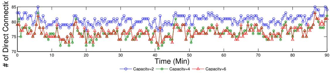
Fig. 6. The number of direct connections to the BS while devices have different maximum connection capacities. Communication range is 10m.
