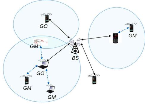
Fig. 1. D2G networks in which heterogeneous mobile devices reside.
