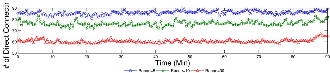
Fig. 7. The number of direct connections to the BS while devices support different communication range
