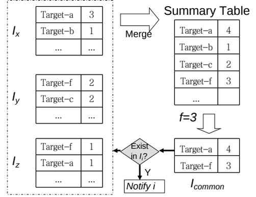
Fig. 2. BS merges information from  $I_x$ ,  $I_y$  and  $I_z$  into a single Summary Table (ST). In ST, only records with counter value no less than 3 are kept, labeled as common interests among these three devices.
