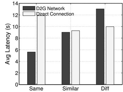
(c) The average latencies comparison when a device is in the D2G versus direct connection
