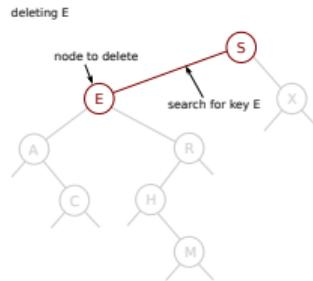
Deletion: to delete a node with key  $k$  (Hibbard deletion),
