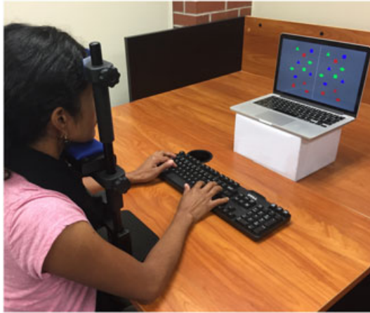
Figure 1. Experimental setup for comparative visual search task. (Note: keyboard shown here differs from the Apple wireless keyboard used in the experiment.)
